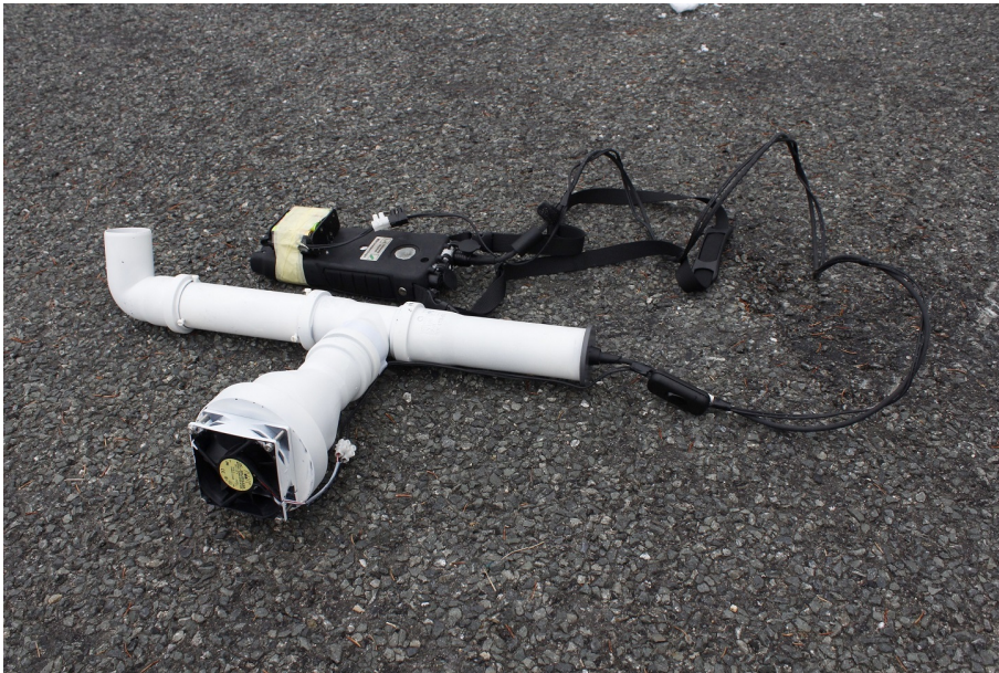
Figure 2.7.: Actively ventilated radiation shield for the mobile thermohygrometer air temperature sensor.
