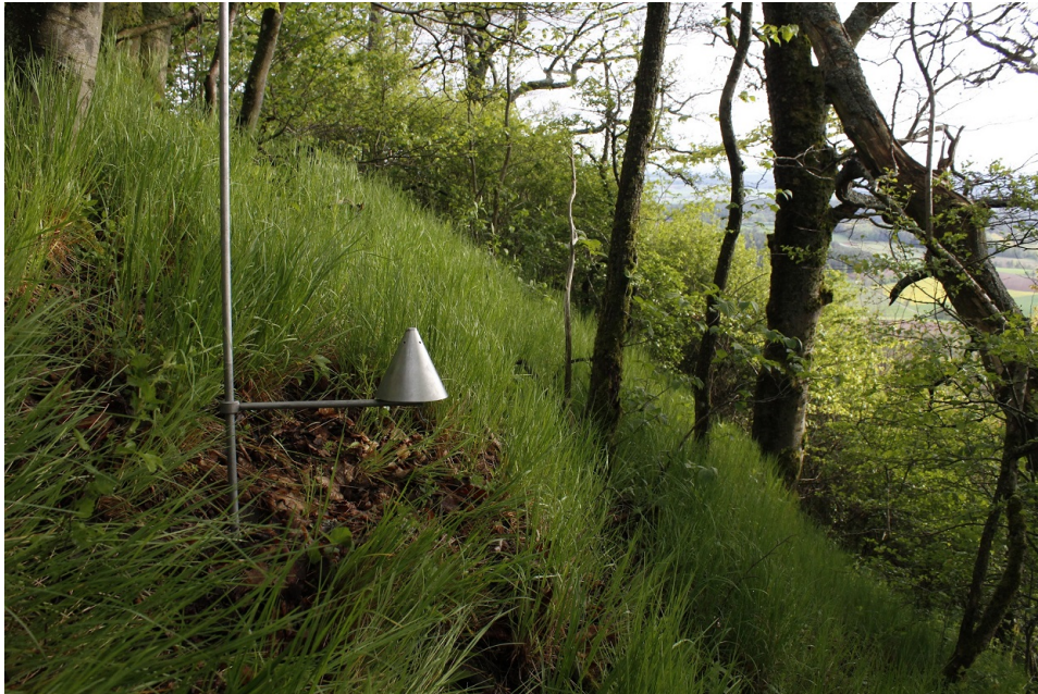
Figure 2.6.: Stationary thermohygrometer at F7 above the block field at Rauher Kulm.
