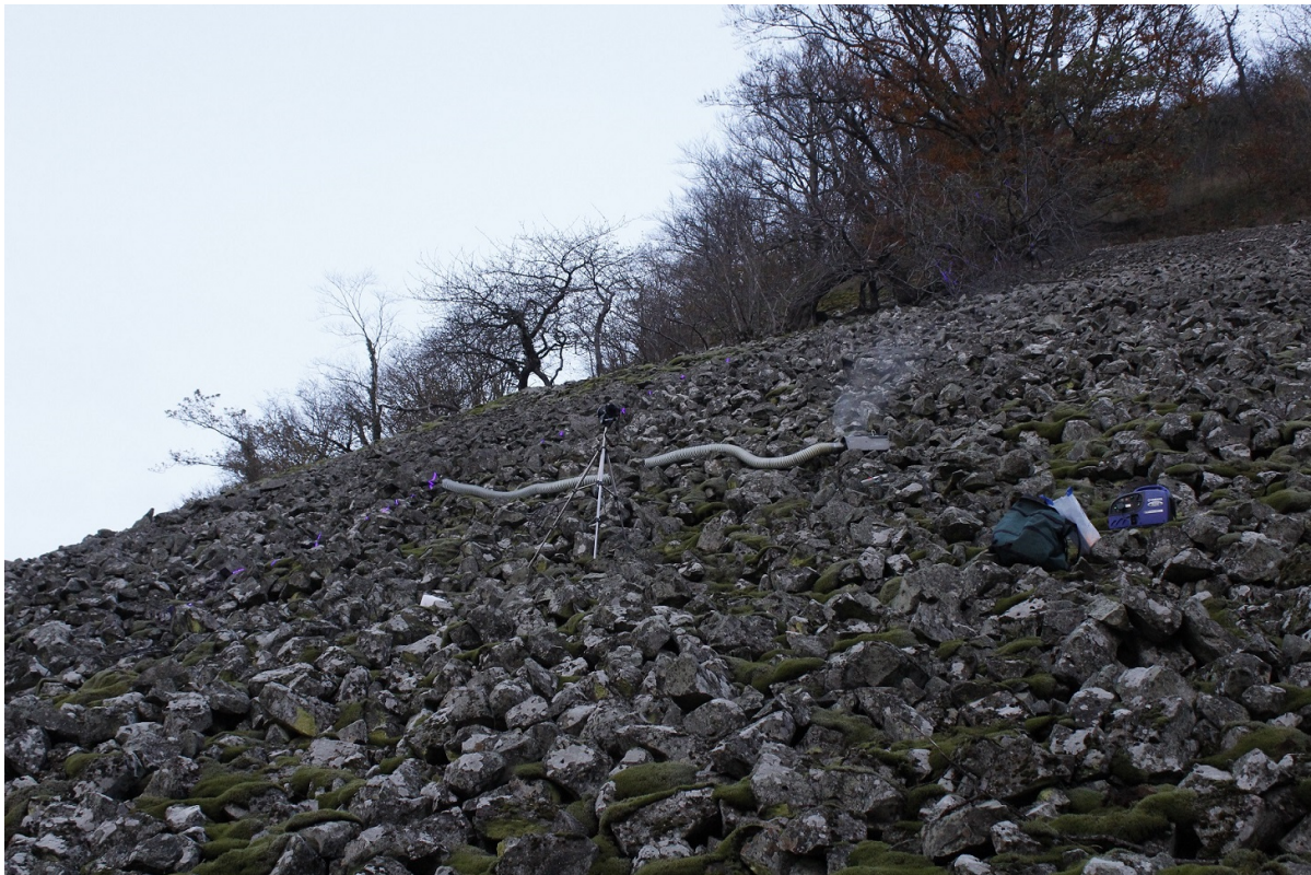
Figure 2.10.: Block field at Rauher Kulm with setup for the flow visualization experiment: Power generator, fog machine, tube for fog locating, camera for documentation (from right to left). The laser was located to the lower left outside of the image.
