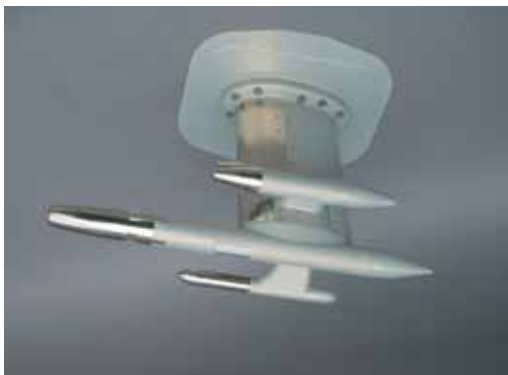
Figure 4: Photograph of the CARIBIC inlet system.
