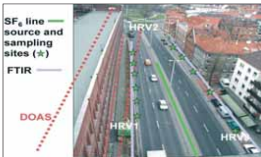
Figure 1: Street Canyon 'Goettinger Strasse with instrumentation. The picture shows the continuous monitoring stations HRV1 to HRV3 (white) and the SF 6 -line-source at the median strip plus the sampling bag locations (green). The path-averaged measurements are indicated by the blue (FTIR) and red (DOAS) lines.
