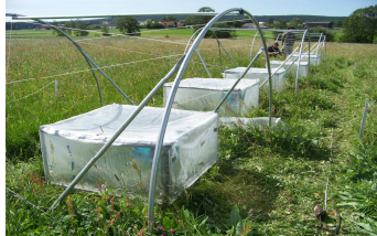
Fig. 3: 13 CO 2 pulse labelling chambers with thermal packs, fans and carbon/acid-reservoirs inside.
