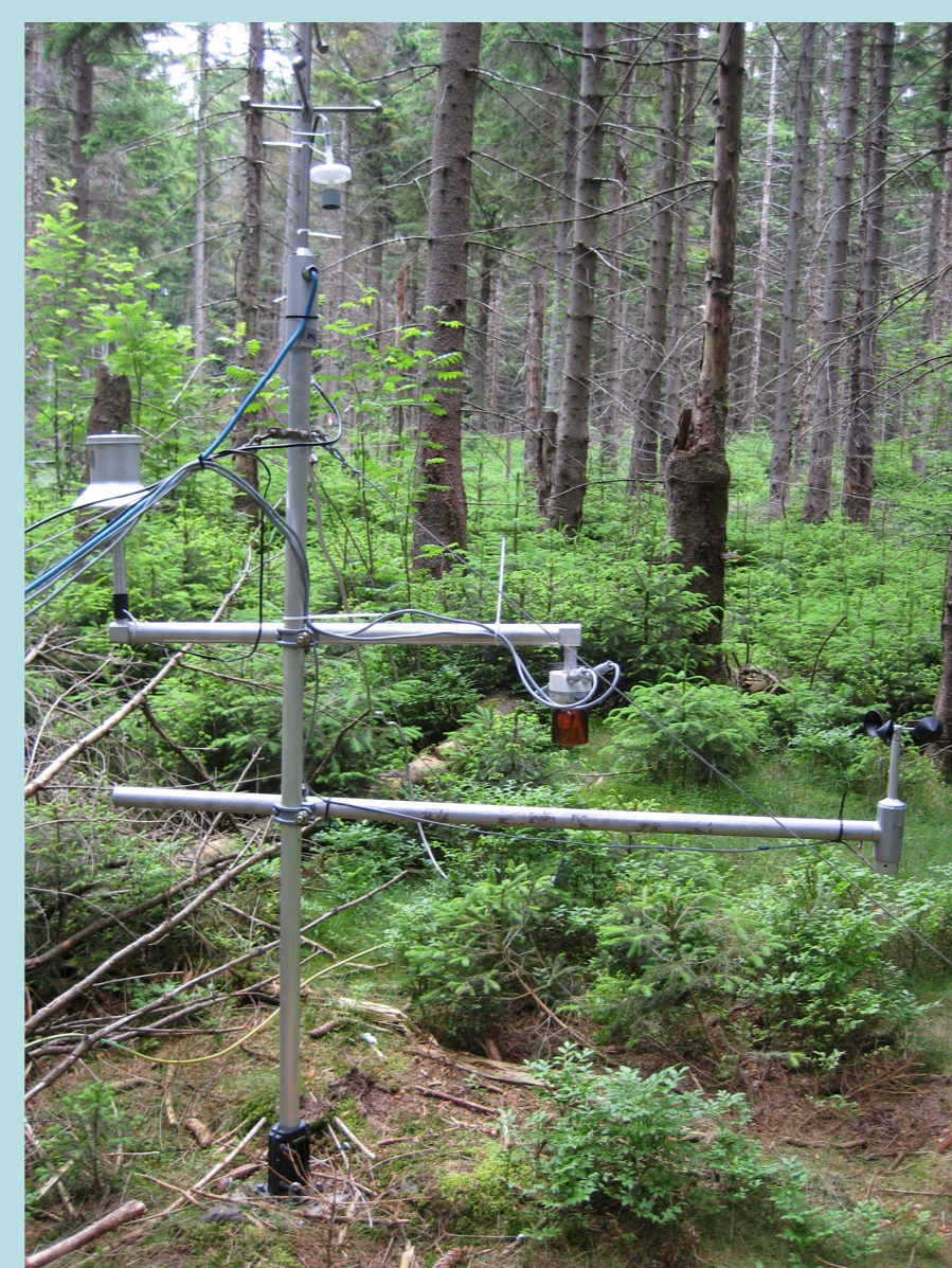
Figure 2: Sub-canopy mast equipped with sonic anemometer USA-1, CO 2 inlet, psychrometer and cup anemometer.
