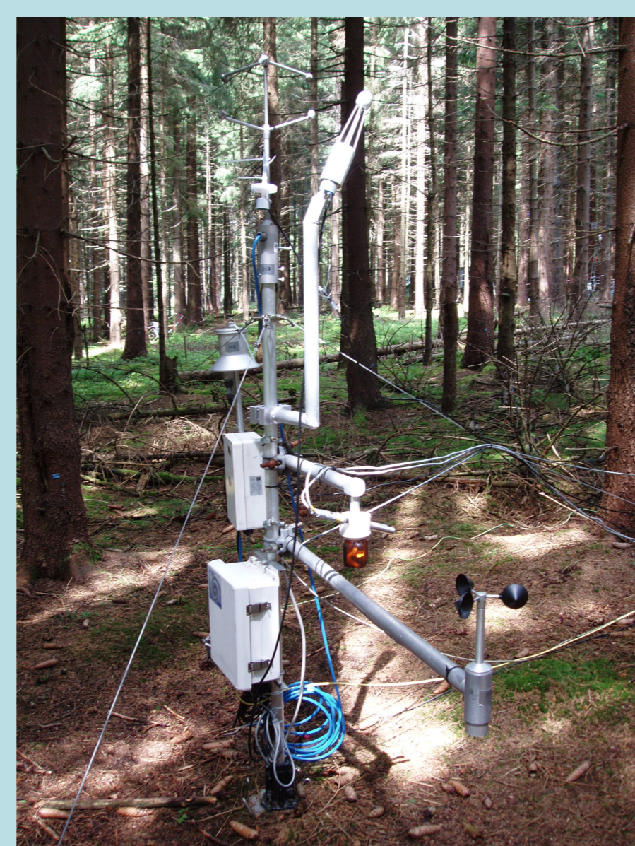
Figure 4: Sub-canopy advection mast equipped with LI-7500 open path IRGA and closed path IRGA inlet for inter system comparison (open versus closed path).
