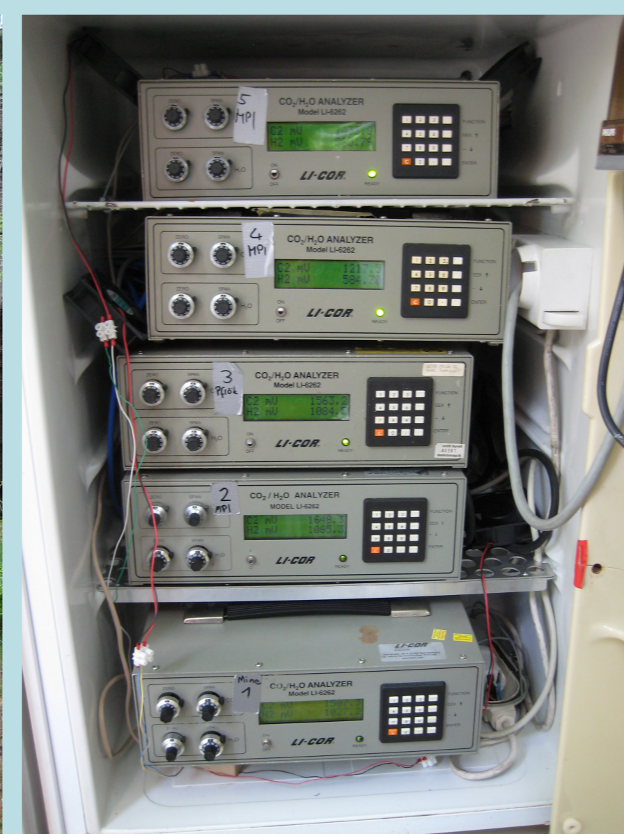
Figure 3: Infrared gas analyzers LI-6262 in a temperature controlled environment.
