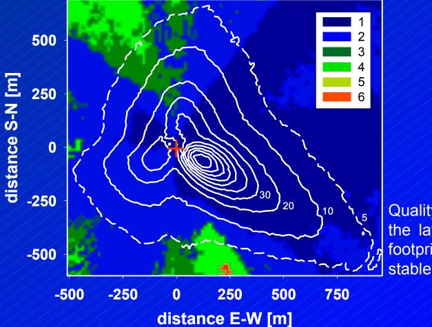
Quality assessment for the latent heat flux with footprint climatology, for stable stratification.
