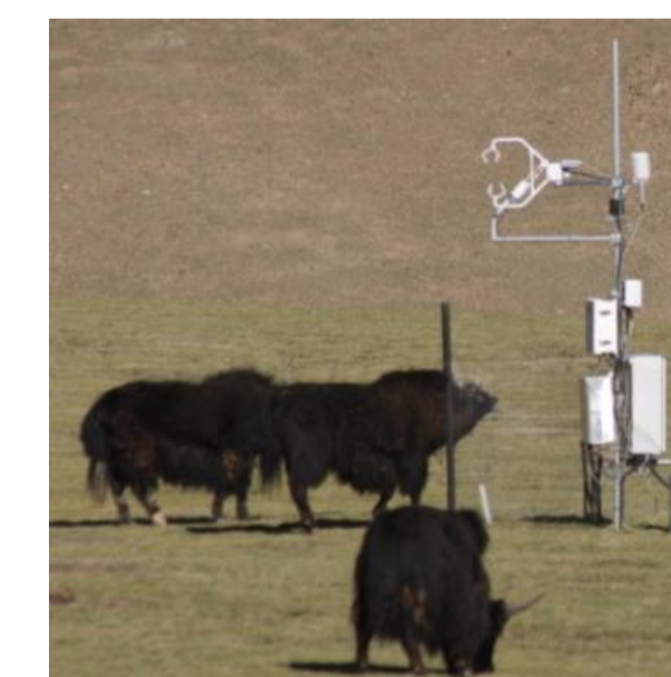
EC-system: sonic anemometer Campbell CSAT-3 and infrared gas analyzer Li-COR 7500
