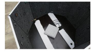
Figure 1.1: antennas of the Minisodar in the experiment set up
